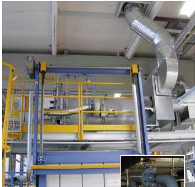
The photo shows a gas-fired furnace for dewaxing with thermal post-combustion, program flow control and temperature regulation using a Siemens-PLC S7 313 with TP 170 touch panel.
